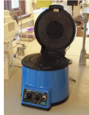
Figure 3: Bullet Blender (Next Advance) was used to disrupt butterfly thoracic tissue to isolate genomic DNA in the Monteiro lab.
