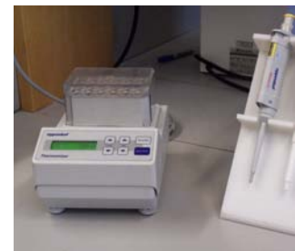
Figure 4: A Thermomixer (eppendorf) was also used to isolate genomic DNA in the Monteiro lab, in preparation for RAD-library construction in the Hoekstra lab.
